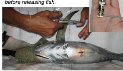
Electronic archival tag with light and temperature sensors at tip of antenna.
