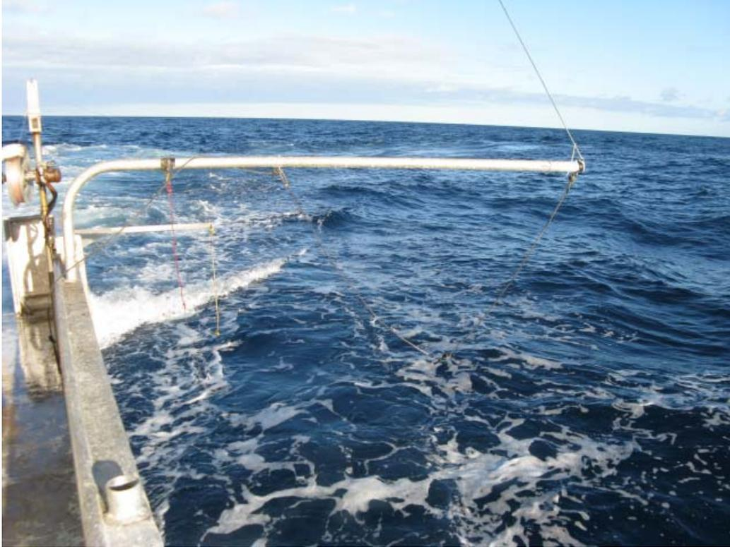
Figure 3. Two dangler poles rigged on the port stern.
