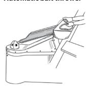
Some large, modern longline vessels use automatic bait throwers. They are generally only seen on larger Japanese vessels. Bait throwers are usually located at the stern of the vessel. They ensure that the bait is thrown well clear of the vessel's wash so it sinks more quickly and without tangling. This is especially important if there is a problem with sea birds.
