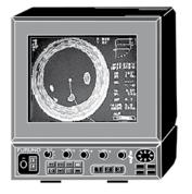
The sonar displays solid objects in the water column below or to the side of the vessel. Sonars are more commonly seen on purse-seine vessels but may also be seen on larger longliners.
