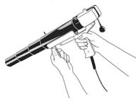
Expendable bathythermographs collect information on the temperature of the water column. Continuous temperature readings are taken by the descending falling probe, thus showing the temperature structure of the ocean. The information is used to find thermoclines, ocean fronts or current eddies that will indicate the presence of fish/tuna.
