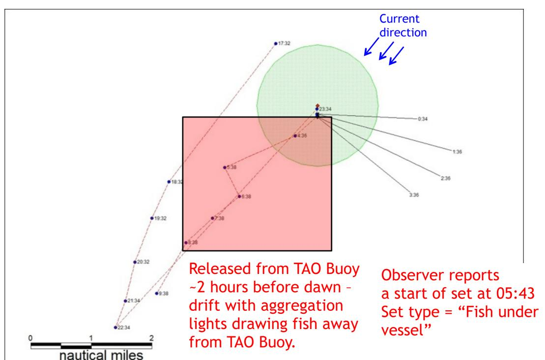
Vessel drift consistent with current direction during set
