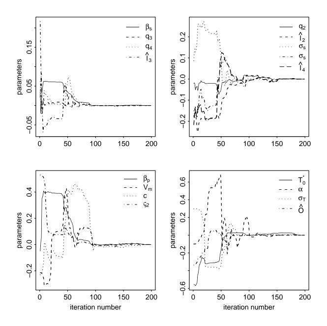
Figure 3.3: Evolution of control parameters during twin data experiment conducted for the artificial data simulated with E2 parameter set. Parameters are grouped by their sensitivities in descending order, except  $\beta_p$  for which high sensitivity was calculated by both SA-1 and SA-2 analysis.
