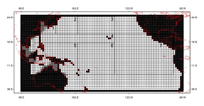
Figure 2.1: Computational domain with 3-layer mask and 2 degree grid (black color - land, dark gray - one vertical layer, light gray - two vertical layers, white - three vertical layers.
