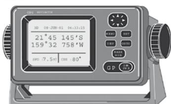
The Global Positioning System (GPS) displays the vessel's exact position in latitude and longitude. The UTC time is also available on the GPS. The GPS will help observers to record positions and UTC times. The use of the GPS should be discussed during the placement meeting.
