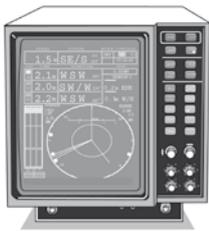
The Doppler current meter displays the direction and strength of the current at various depths. The current's strength is displayed in knots and the current direction is displayed in degrees.
