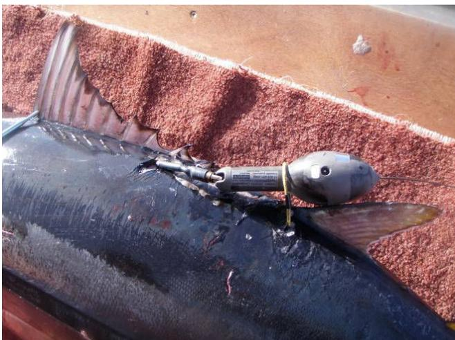
**Figure 2:** A miniPSAT fitted on an albacore tuna to test tag attachment. Two anchors hold the tag. Before placing it on the fish, it is programmed to self detach after a programmed time and/or depth. Data are transferred to satellite when the tag pops up.
