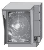
A bird radar is equipped with a large coloured screen. It displays the presence of small items that cannot normally be seen with the navigational radar. This includes flocks of birds, which may be a sign that there is a school of tuna present.
