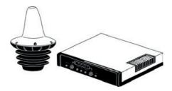
The VMS (vessel monitoring system) tracks the vessel's position using satellite technology and relays the position to a monitoring station on shore. This signal is transmitted to a satellite. Observers should be able to identify the MTU (mobile transponder unit) box or 'black box' in the wheelhouse. The box may send out a beeping sound at constant intervals, but this can be turned off. (Often a silver seal with individual numbers seals the sides of the MTU, although observers are no longer
