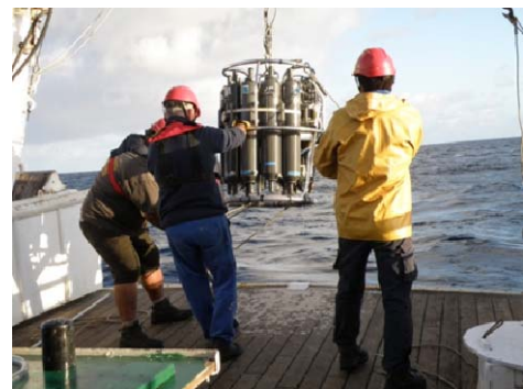
Recovering the CTD probe and the sampling water bottles
