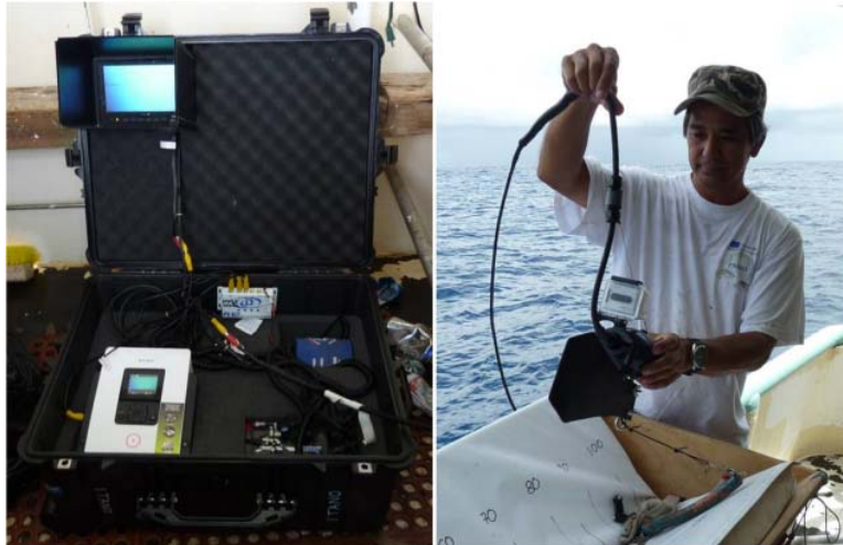
Figure 17. SplashCam recording and viewing system (left) and camera head with GoPro Naked video camera attached (right)
